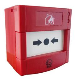
It has been designed according to EN IEC 60079-0:2018, EN 60079-11:2012 and EN ISO/IEC 80079-34:2020 standards as intrinsically safe (I.S) for use in hazardous environments. It also meets the requirements of the EN 54-11 standard. It is a Type A class product that gives a direct alarm when the operating point is pressed.
